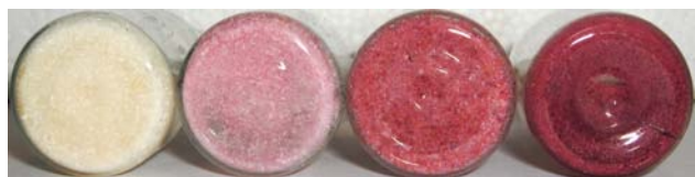
Figure 4. Photograph of the coordination polymers ^3_\infty[\text{Zn}_{1-x}\text{Co}_x(\text{tdc})(\text{bpy})] in dependence of their \text{Co}^{2+} content; from left to right: increasing cobalt content, x = 0; 0.1; 0.5 and 1.0 .
